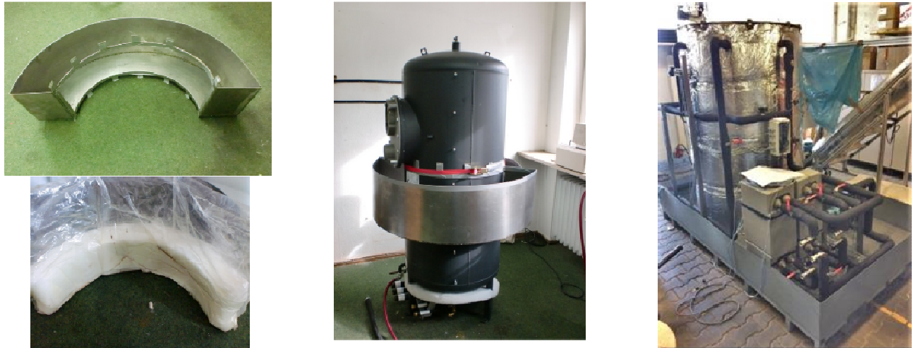
Fig. 2: Examples for active storages in the water heating circuit.
