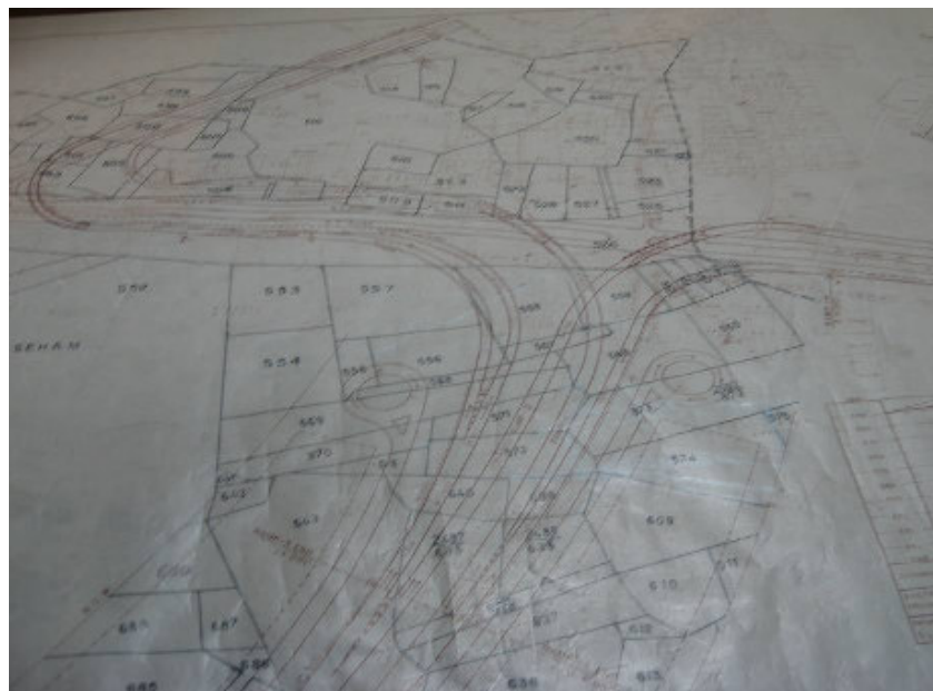
Figure 5. Proposed Ring Road II Plan overlaid on cadastral map for land acquisition planning
