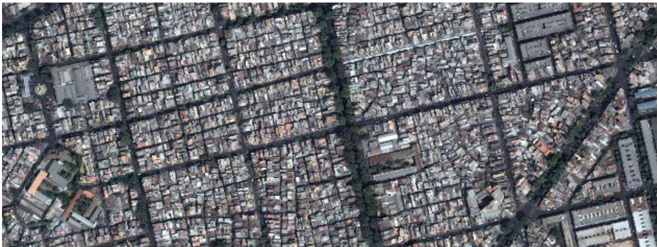
Fig 16. Compact urban structure of HCM City with shophouses as the basic module (Quickbird 2005)
