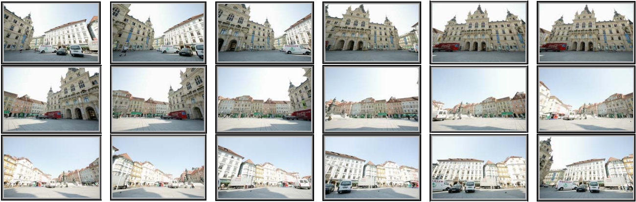
Figure 2: Collections of 18 source images (4064x2704) taken in front of the city hall with an angular separation of 20°.
