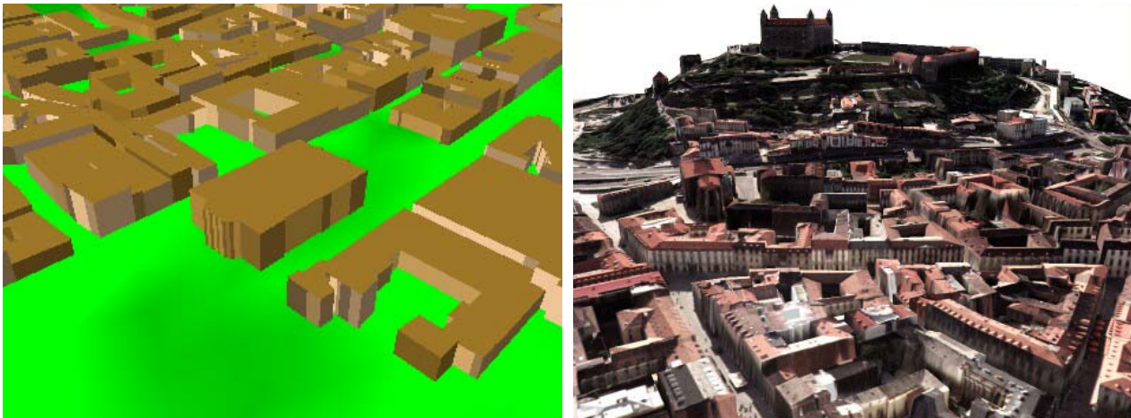
Figure 10: Flat-roofed building block models made from the footprints and the city visualization. The only one exception in the right picture is a castle surrounding, made from the roof plans from the Figure 8, all the other buildings are flat-roofed.
