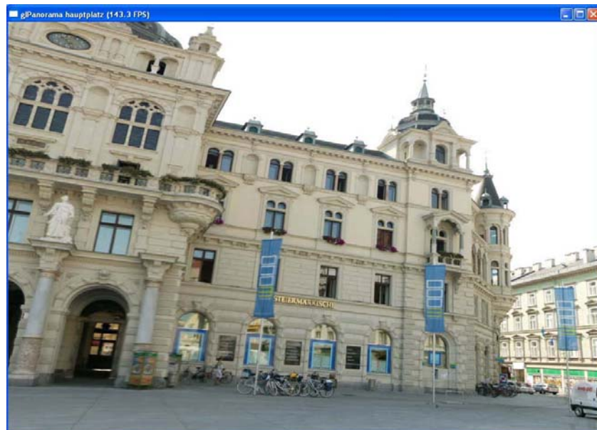
Figure 6: Visualization of a 14000x2704 high resolution panorama covering the main square in front of the city hall. We obtain a frame-rate of 70-100 frames/sec on a 1,6 GHz Intel processor with 512MB main memory and a GeForce4 with 64 MB graphics memory.
