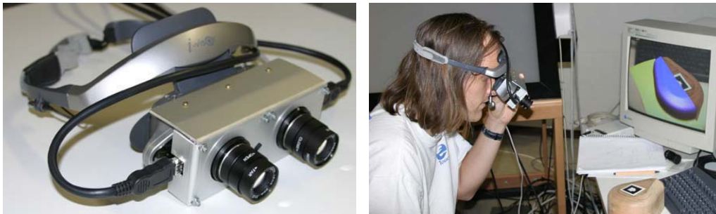
Abb. 1: Augmented Reality HMD Cy-Visor. [Quelle: HLRS, 2003]
